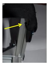
Toe-strap tie helps hold the toe strap in place
