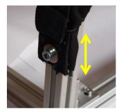
Allen bolt fixing to upright allows additional adjustment of toe strap
