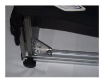
Right-angled bracket added to reinforce the up-right to prevent possible fatigue failure of lower rail
